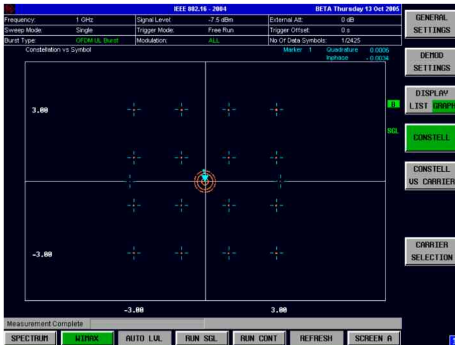
Fig. 90 IQ imbalance influence on the unallocated carriers using subchannel index 4
