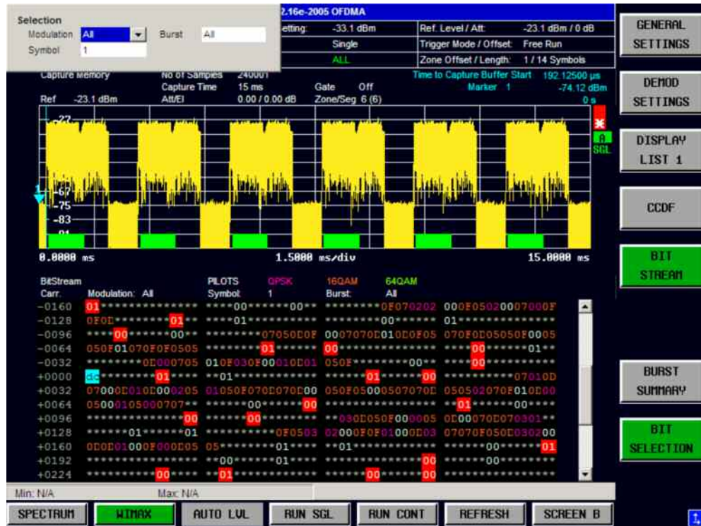
Fig. 34 Bit-Stream for OFDMA, showing the Bit Selection dialog and highlighted pilot errors.
